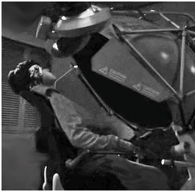
Figure 2: Satoru’s interface for control. He is visually immersed in the remote environment when looking at the hemispheric display. Satoru’s head has a roll/pitch/yaw motion capture device. Image © 2005 Hinokio Film Venturer
