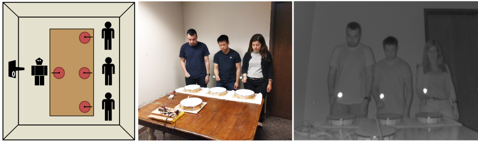
Fig. 2. Left: Experimental setup. A Kinect 2 tracks participant motion, as do piezoelectric sensors in the drums. The robot uses these sensor data to decide when to hit its drum. Center/Right: Three participants drum with the robot during a pilot study. RGB and IR images are shown.
