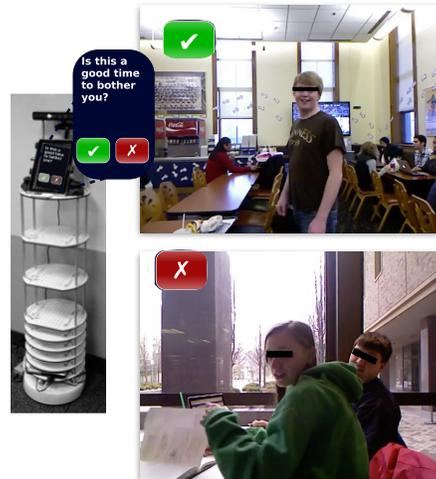
**Fig. 1:** A robot approached hundreds of participants in real-world settings, asking for permission to interrupt them. An on-board Kinect captured RGB-D and audio data. Two images are shown from the robot's perspective: in the dining hall where a participant agreed to be interrupted, and in the library where participants declined.
